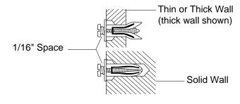
Figure 6 - Tightening Anchors
